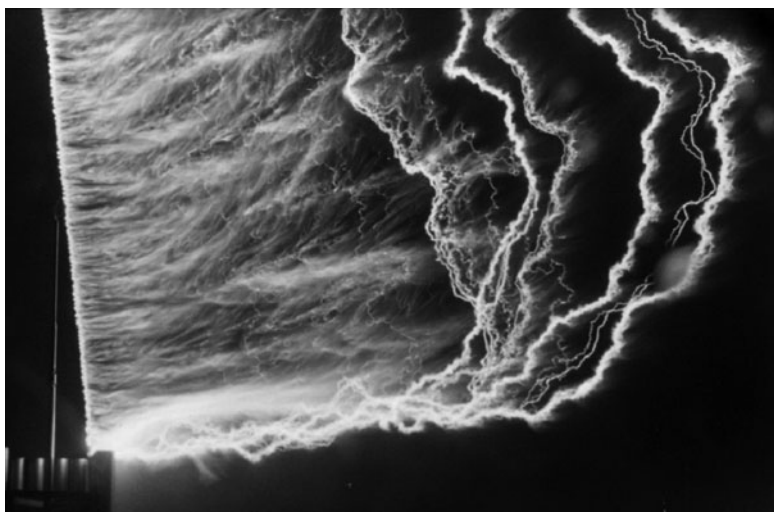
Figure 7.7 Rocket triggered lightning. A first stroke follows the copper wire trailing the rocket. Successive strokes follow the conductive path blown away by the wind (from [21]).
